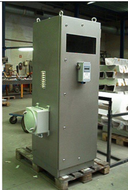
19 «rack cabinet for analyzer
